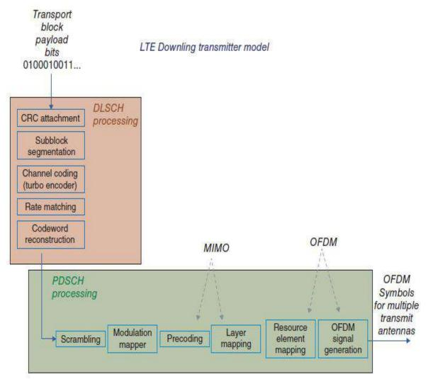
Fig. 2 Physical Layer Specifications in LTE
