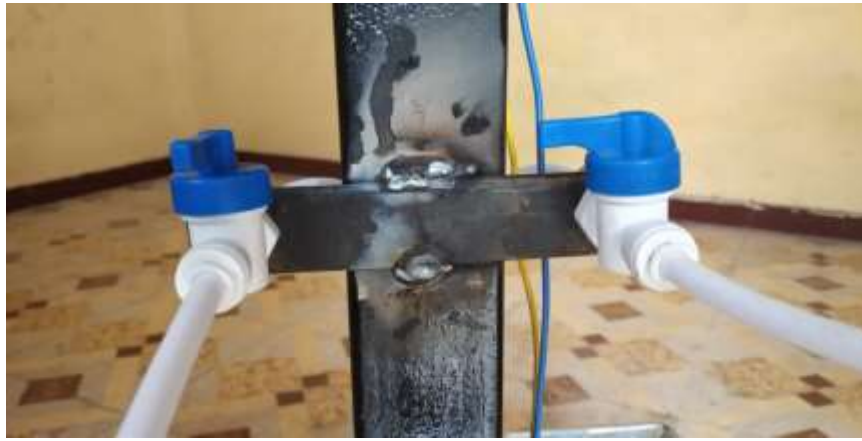
Fig. 7. Flow Control Valves
