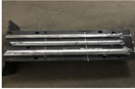
Figure 8: Al-SiC composite sample for shaft
