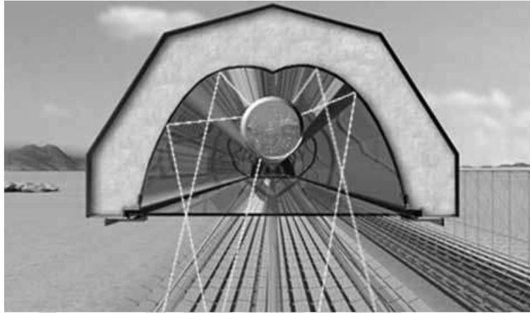
Figure 2. A secondary Trombe-Meinel cusp concentrator [4].
