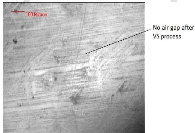
Fig. 4 Microscope image after the VS process
