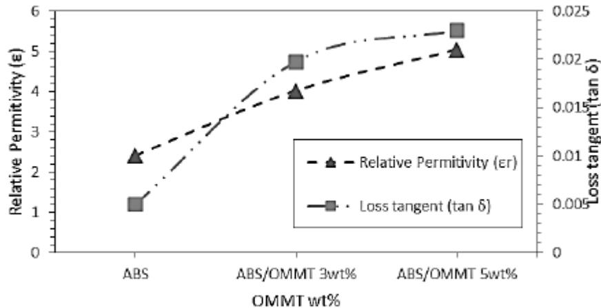
Figure 3 relative permittivity and loss tangent
