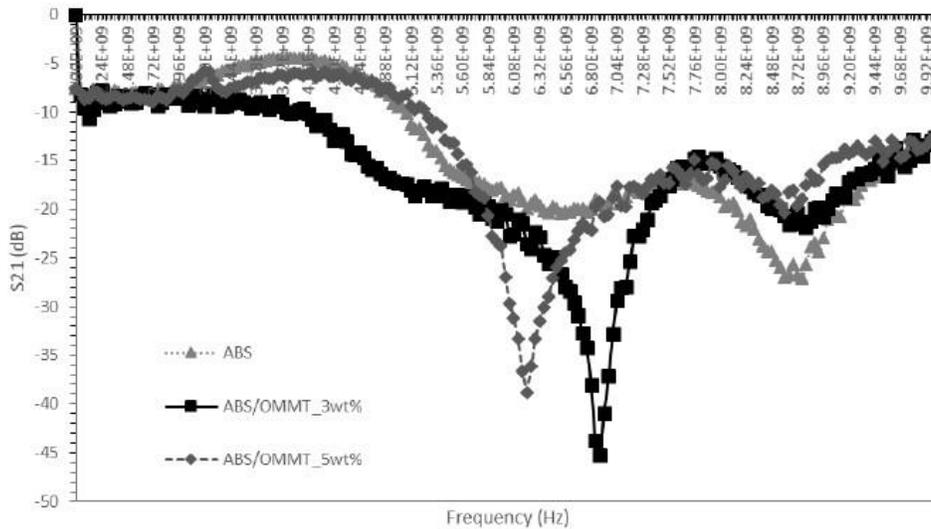
Figure 2 S21 vs frequency plot for tee resonator
