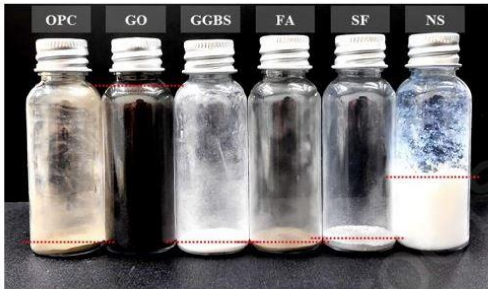
Figure 2. Differences in Volume among Samples with the Same Amount (5 G) Of Additive.
