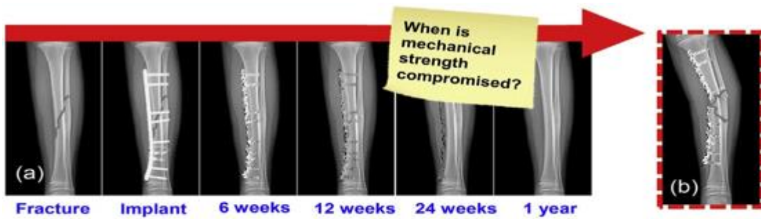
Figure 1. Schematic Representation of (a) Normal Degradation of a Plate/Screw Construct in One Year and (b) Premature Catastrophic Failure Due To Stress Shielding and Stress-Corrosion Cracking.
