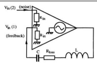
Figure 1. Equivalent circuit model of oscillator
