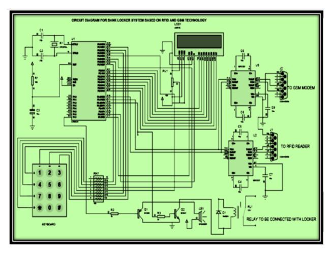
Fig.2: The Figure Shows the Circuit Diagram of the System
