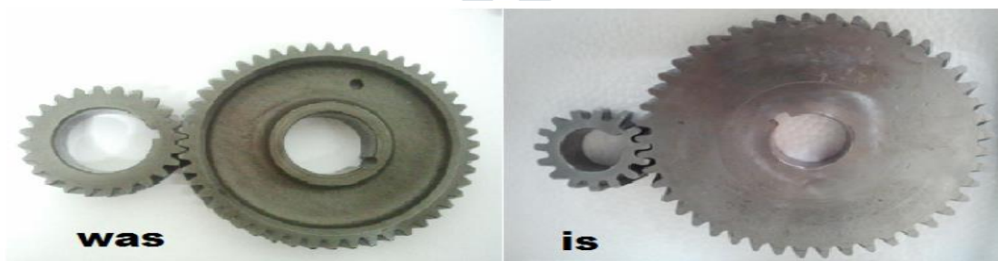
Figure 3: Shows the old cam and crank shaft gears used in the 4- stroke engine and the same gears now being used in the 6-stroke engine
