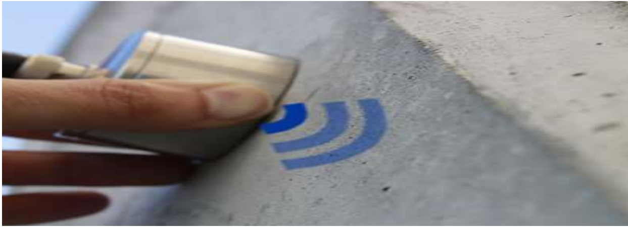
Fig. 7 UPV test on concrete
