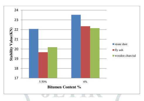
**Marshall Stability graph:** Maximum stability value of 23.53 KN is observed at 6% bitumen content in case of stone dust as a filler.
