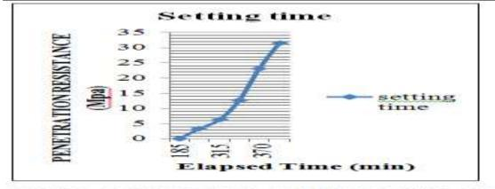
INITIAL SETTING TIME CORRESPONDING TO 3.5 MPA RESISTANCE = 278 MIN
