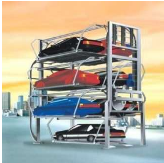
Fig.4 Rotary parking system
