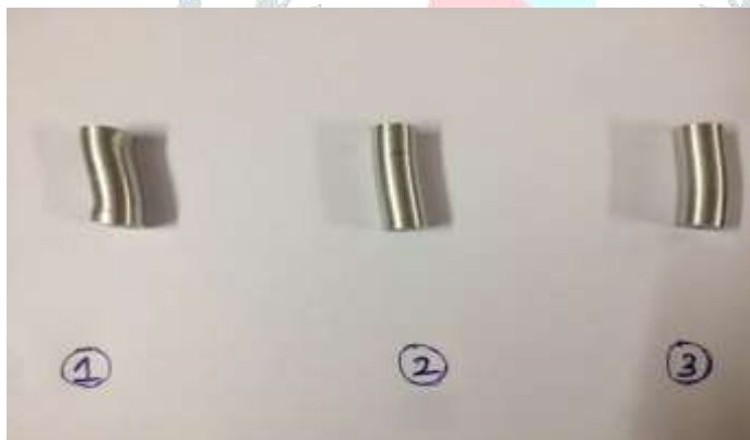
Fig.3.2 Compression Tested Specimen. (1) 1wt% NanoSiC (2) 2wt% NanoSiC (3) 3wt% NanoSiC
