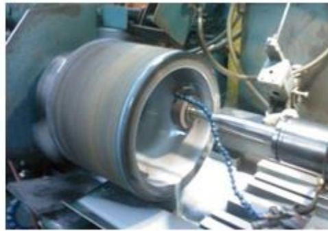
Fig. 6: Chunking Type Internal Grinding
