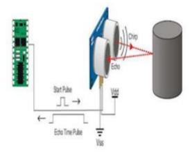
Figure 1: Detection Principle of Ultrasonic Sensor
