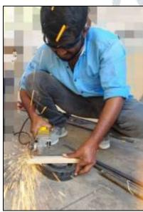
Fig 11. Cutting Operation performed on Square pipe
