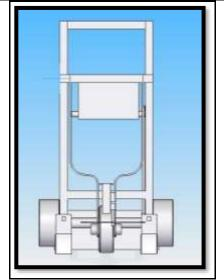
Fig 1. Assembled and Modelled in Solid Edge V19
