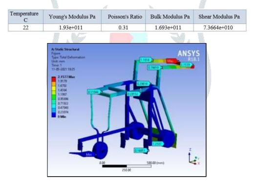
Fig 5. Total Deformation when subjected to load
