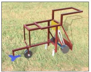
Fig 10. Assembled And Rendered Modeled (Iso-metric view)
