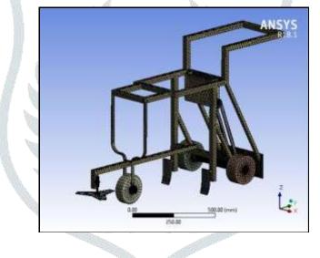
Fig 3. Meshed model in Ansys 18.1
