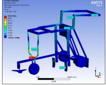
Fig 6. Von- Mises stress Acting on the body
