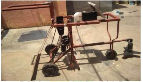
Fig 16. Completely assembled multipurpose seed sowing machine
