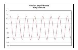
Fig 7. Constant amplitude cycle graph
