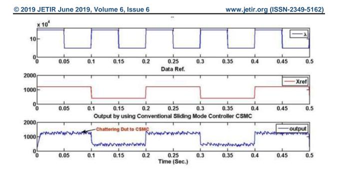
Figure 5: Output rate of the proposed system
