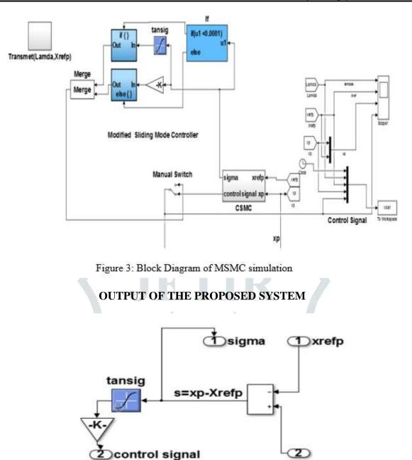
Figure 4: Simulation of sliding mode controller
