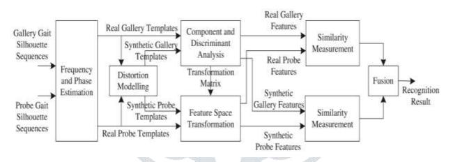
Fig. 1: Diagrammatic View of human recognition via presented statistical feature fusion approach
