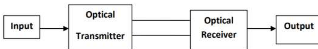
Fig 1 Generic Optic communication system
