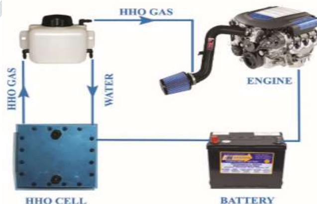
Fig 2: working of hho generator.
