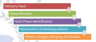
Sensors - ultrasonic and accelerometer are used to collect data. This data is then assigned to specific variables and these variables are then used to calculate gait phase position (stance or swing phases), gait mode (walking, jogging, or running). This information about the gait phase and mode is then used to calculate the suitable damping for the prosthetic ankle.
