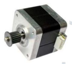
A stepper motor is a brushless DC electric motor which divides its rotation in several steps. The motor's position can then be commanded to move and hold at one of these steps without any position sensor for feedback, as long as the motor is carefully sized to the application in respect to torque and speed.
