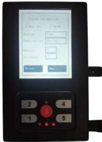
Fig. 4. Programmed POS Device using LPC1768 controller
