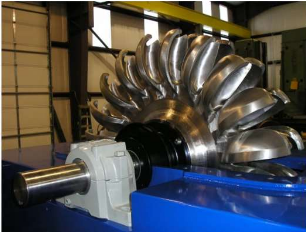
Fig. 1: Illustrates the pelton wheel turbine used to convert hydraulic energy in to kinetic energy.
