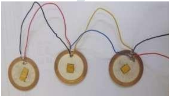
Figure 4. The series connection of piezoelectric transducer
