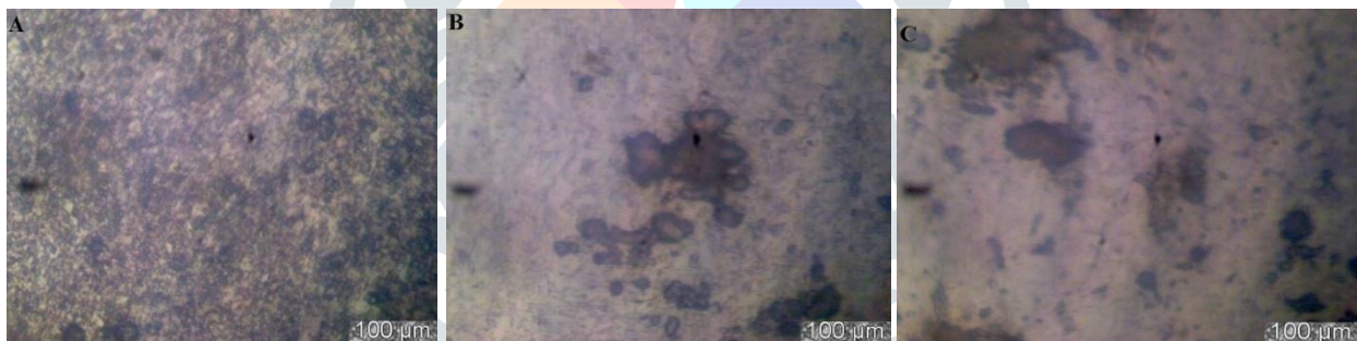
Figures 5. (a) Optical micrograph showing the microstructure of sample heated to 750°C held for 30mins, (b) Sample heated to 750 °C held for 1hr, (c) Sample heated to 750 °C held for 2h.
