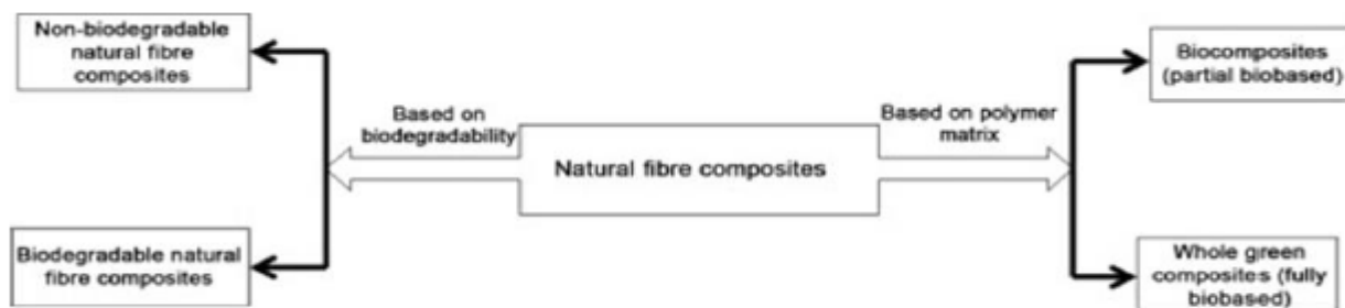
Figure 4 Basis of classification of Natural fibre Composites
