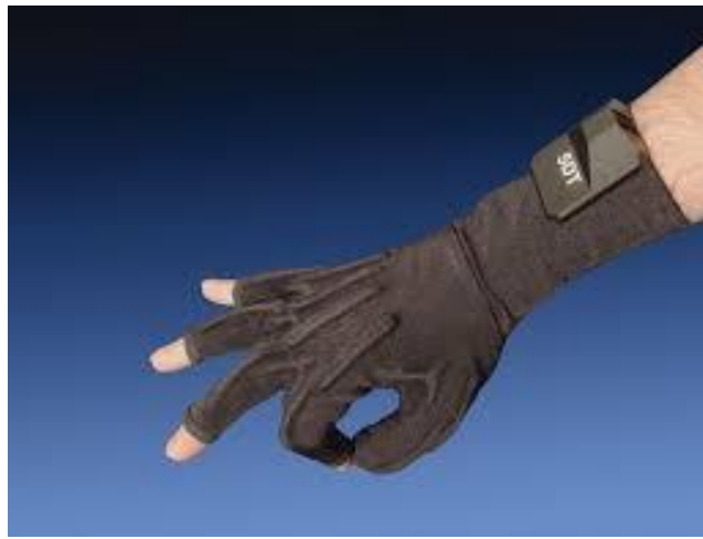
Figure 3: Illustrates the module of Data glove with sensors[6]
