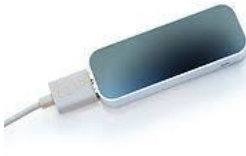
Figure 1: Illustrates the leap motion controller with USB[4]
