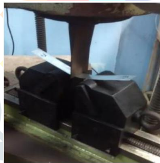
Figure 4 Flexural Specimen Setup in Universal Testing Machine
