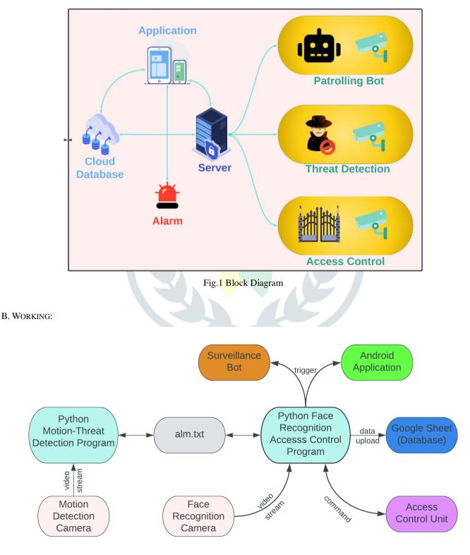
Fig.2 Hardware and software working setup
