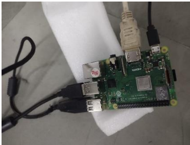
Fig. 2 Hardware connections with Raspberry PI 3B+
