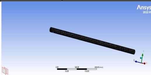
Fig.35:Meshing on Column
