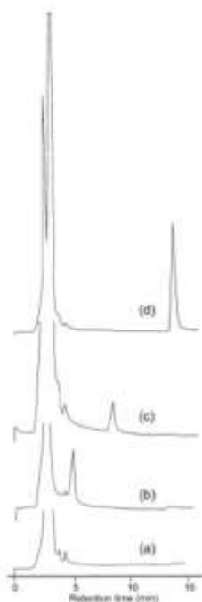
Fig. 4 Typical HPLC chromatograms of toddy, (a) without adulteration and containing, (b) CHL, (c) ALP and (d) DIA.
