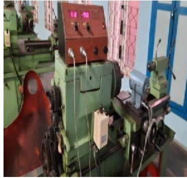
Figure4.5:Tool Dynamometer set up with lathe machine
