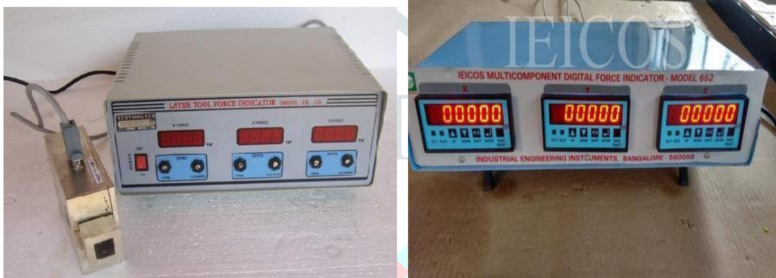
Figure 4.1: Lathe Tool Dynamometer to Measure Cutting Force
