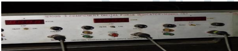
Figure 4.2: Digital panel meter Operation of Lathe Tool Dynamometer with Multi Component Force Indicator
