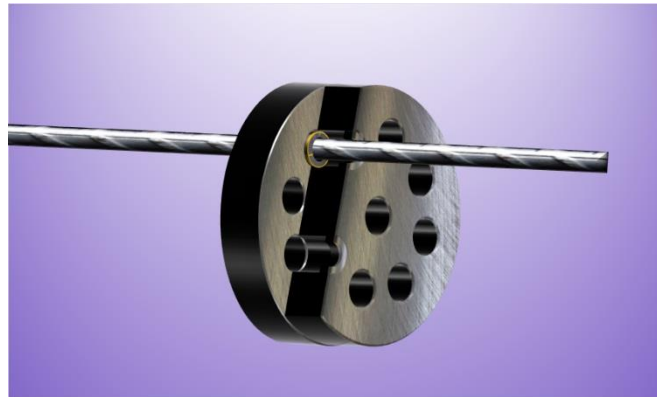
Fig. 3 Modified Freyssinet prestressing system
