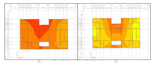
Fig. 5 Rotational Displacement in X and Y direction
