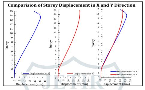
Fig. 4 Comparison of Storey Displacement
