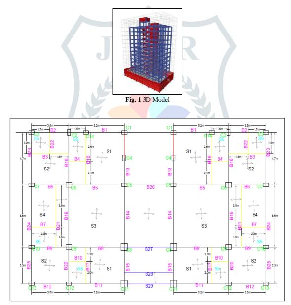
Fig. 2 Structural Plan
