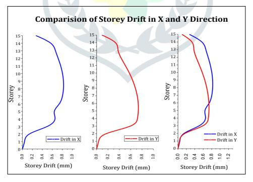
Fig. 3 Comparison of Storey Drift
