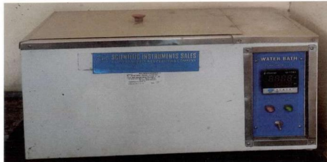
ASPHALT WATER BATH
