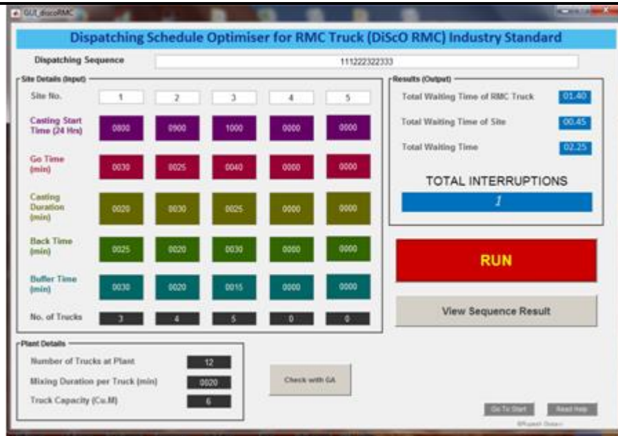
Fig.1 Result of MATLAB App for Case 1 with industry logic
