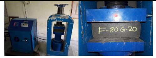
Fig.8 Compressive testing of Geopolymer Brick RESULTS AND DISCUSSION
