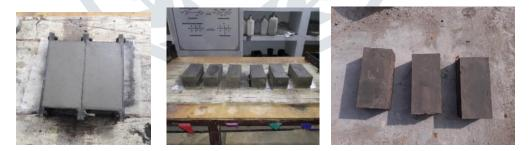
Fig.5 Bricks in Mould Fig.6 Geopolymer Bricks Fig.7 Ambient Curing
