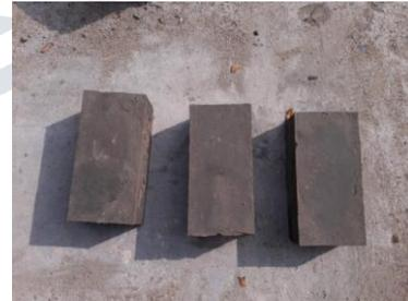
**Fig.5 Bricks in Mould Fig.6 Geopolymer Bricks Fig.7 Ambient Curing**
