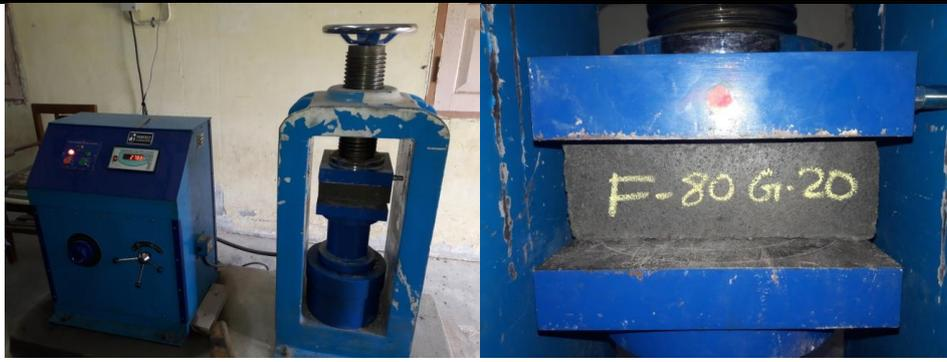
**Fig.8 Compressive testing of Geopolymer Brick**
