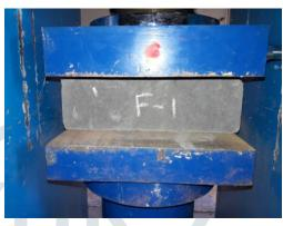
**Fig.4 Fly Ash Brick**
