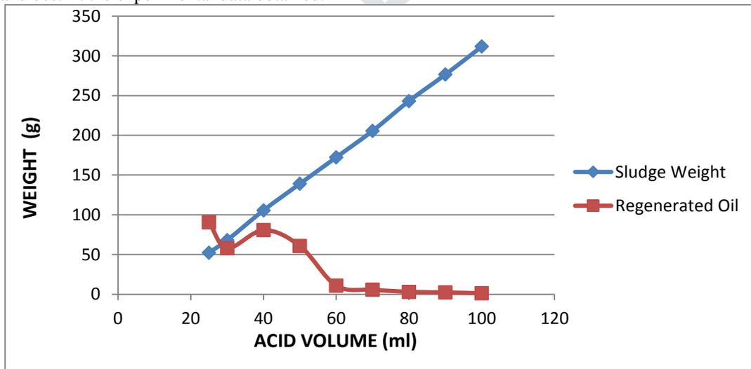
Fig 1 Variation of Sludge and Oil Weight with Acid Volume
