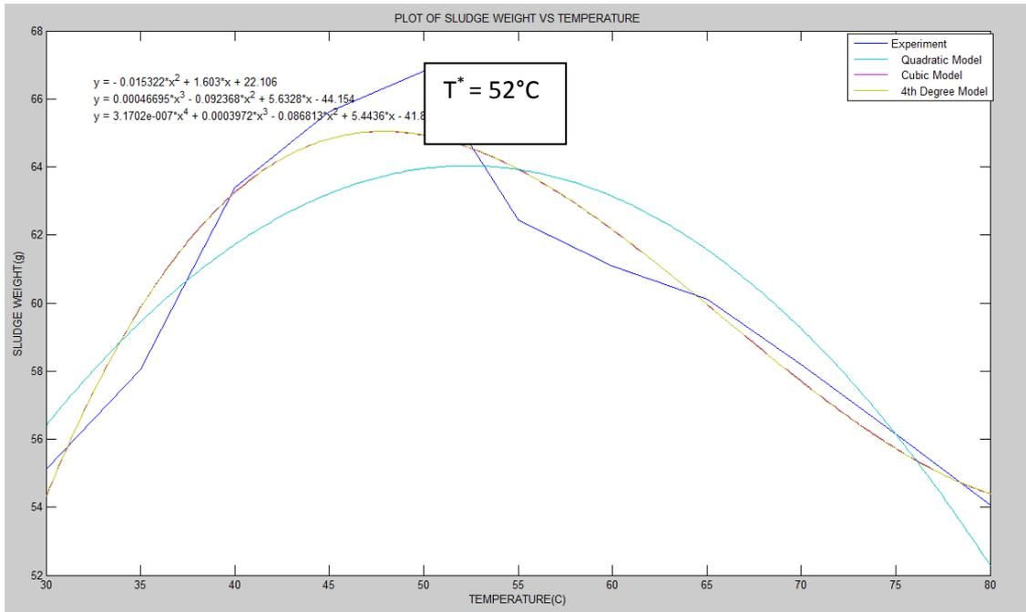
Fig. 3 Effect of temperature variation on sludge weight
