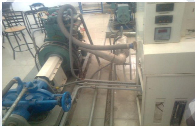
Figure 2. 2 cylinders, 4 stroke diesel engine test setup
