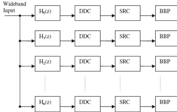
FIGURE 1: PER-CHANNEL APPROACH BASED CHANNELIZATION
