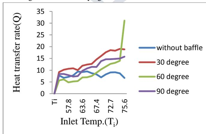
Graph 8.5 Q Vs  $T_i$  at different angles when mass flow rate is 0.06 kg/s
