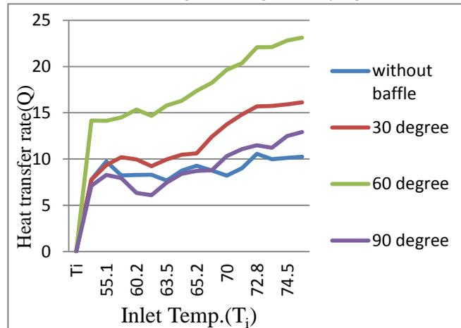
Graph 8.6 Q Vs  $T_i$  at different angles when mass flow rate is 0.05 kg/sec
