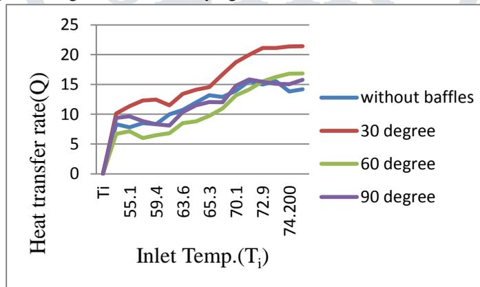
Graph 8.4 Q Vs  $T_i$  at different angles when mass flow rate is 0.07 kg/s
