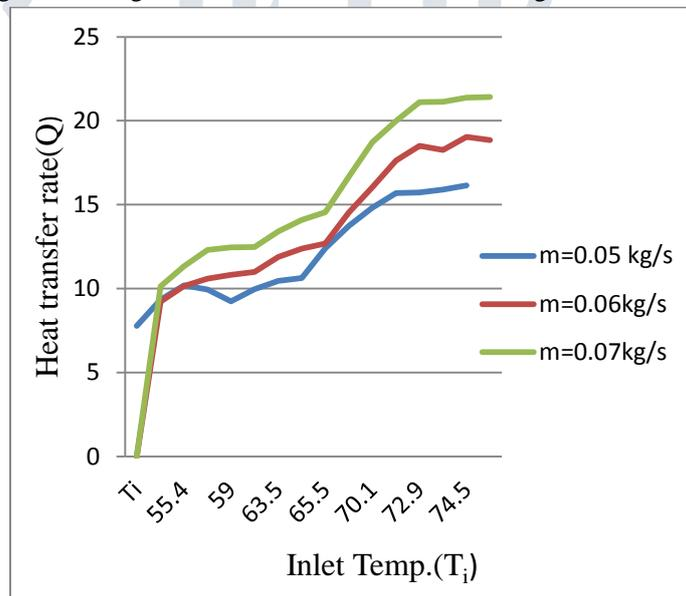
Graph 8.1 Q Vs  $T_i$  for different mass flow rate when baffles are oriented at  $30^{\circ}$
