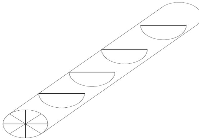
Fig.4.1 Schematic of half circle baffled tube
