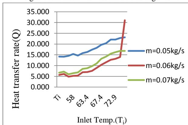
Graph 8.2 Q Vs  $T_i$  at different mass flow rates when baffles oriented at  $60^\circ$
