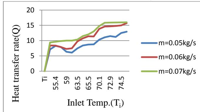
Graph 8.3 Q Vs  $T_i$  at different mass flow rate when baffles are oriented at angle  $90^\circ$
