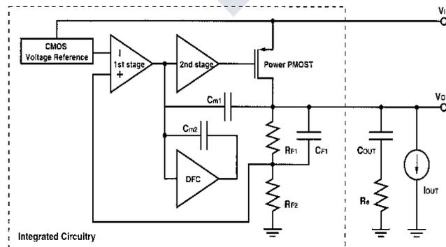
Fig 4: A capacitor-free CMOS low-dropout regulator with damping-factor-control frequency compensation
