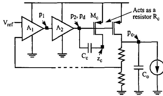
Fig 5: Pole-zero tracking frequency compensation for low dropout regulator.
