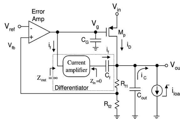
Fig 2 LDO topology with differentiator for fast transient path.
