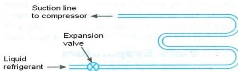
**Fig. Bare Tube Coil Evaporators**
