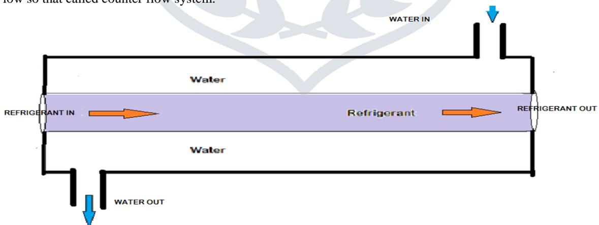
**Fig. Water Intercooler**
