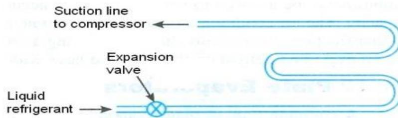
**Fig. Bare Tube Coil Evaporators**
