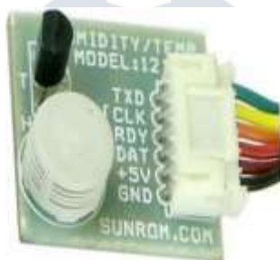
Figure3: Temperature Humidity Sensor
