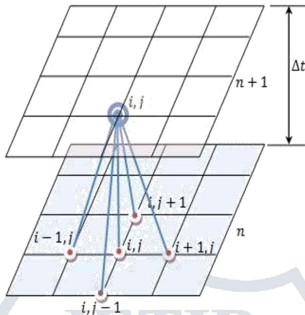
Figure 2: Iterative Procedure for 2-D.
