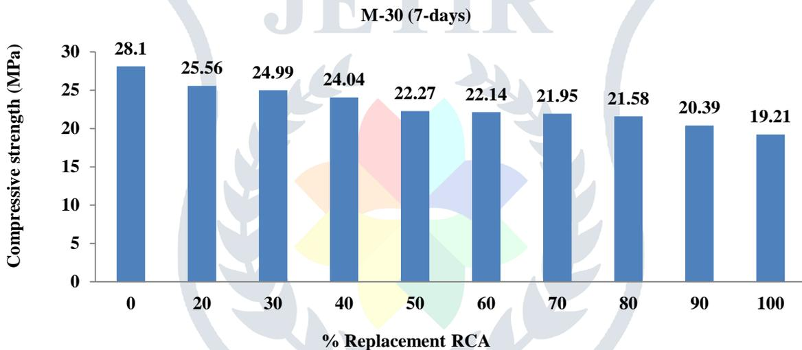
Fig 5: 7-days Compressive strength of M-30 mix concrete with different replacement level of recycled aggregate.
