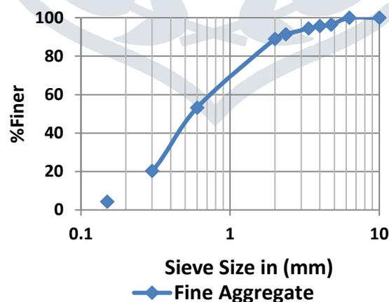
Fig 2: Particle Size Distribution of Fine Aggregate (Natural Sand)
