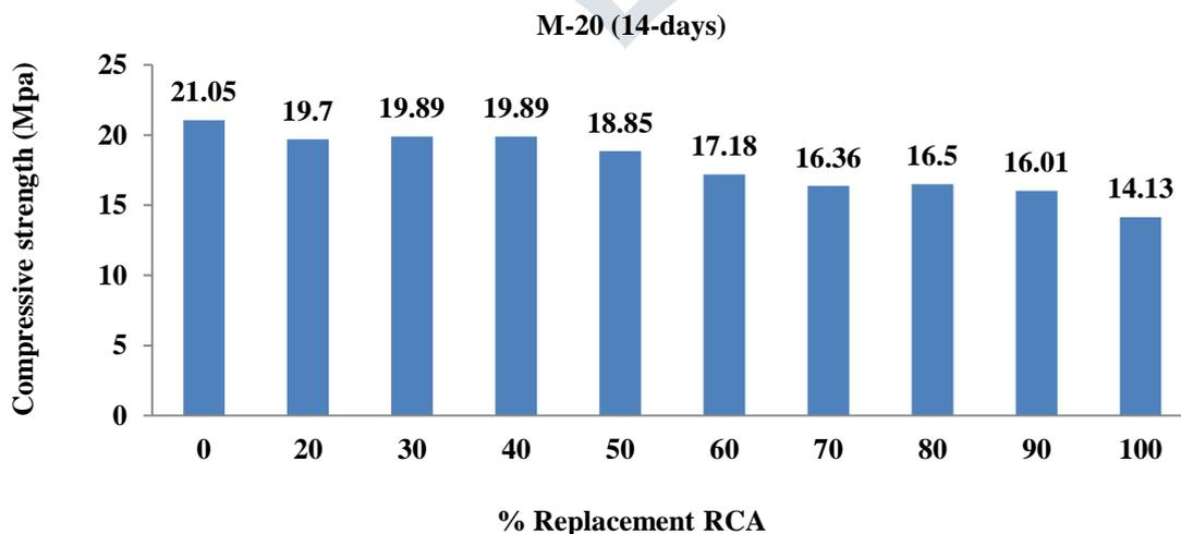
Fig 6: 14-days Compressive strength of M-20 mix concrete with different replacement level of recycled aggregate.
