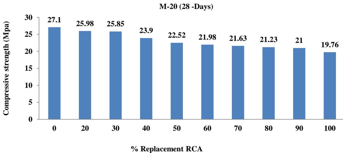
Fig 8: 28-days Compressive strength of M-20 mix concrete with different replacement level of recycled aggregate
